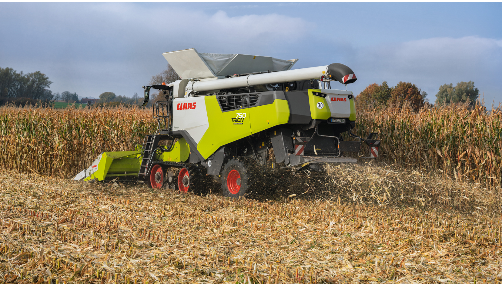
First corn picker with integrated stubble cracker
