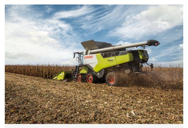
TRION 740, TRION 740 TERRA TRAC and TRION 740 MONTANA extend the CLAAS combine harvester range in Europe with compact, powerful hybrid machines with the APS HYBRID threshing unit and ROTO PLUS single rotor.
