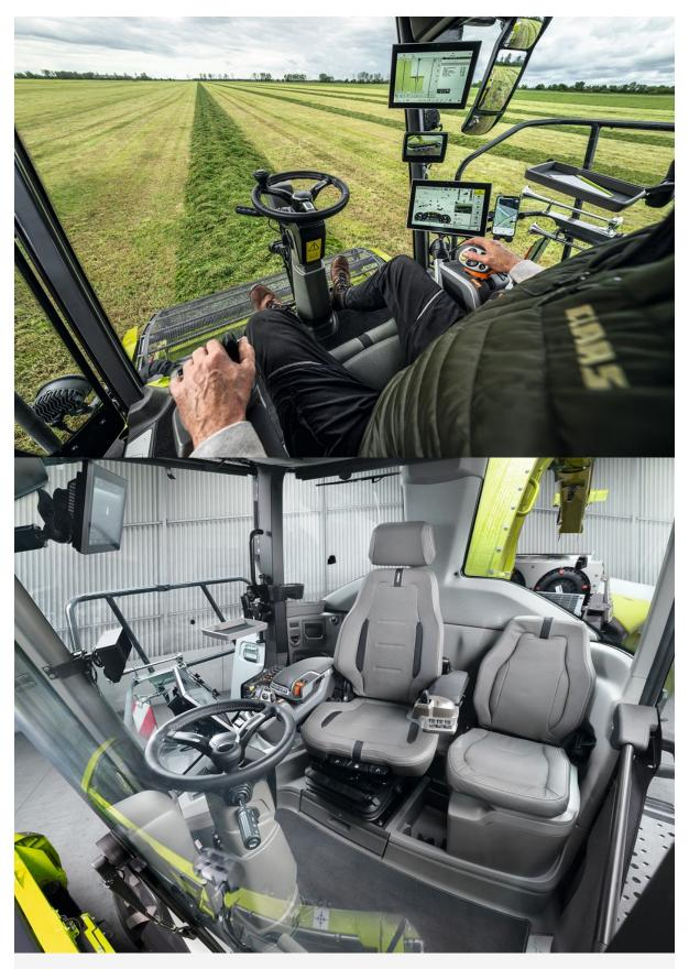
The redesigned cab sets new standards in all-round visibility and noise levels. For the first time on CLAAS harvesting machinery, joystick steering with two steering modes and adjustable intensity levels is available.
