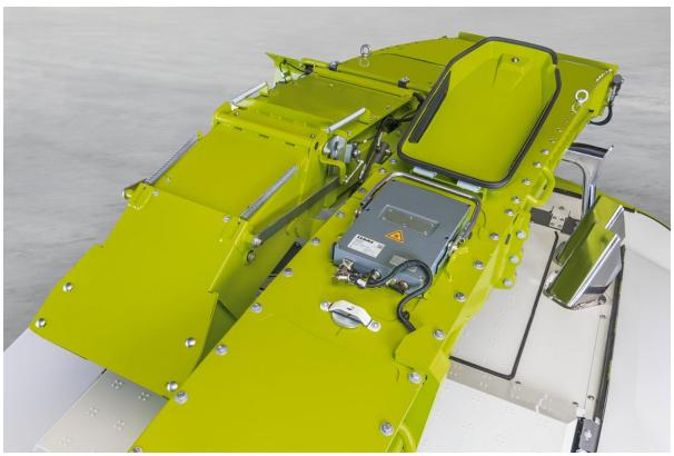
With the JAGUAR 1000, CLAAS is introducing the new NUTRIMETER for the real-time determination of dry matter content and constituents, as well as precise yield recording and yield mapping.
