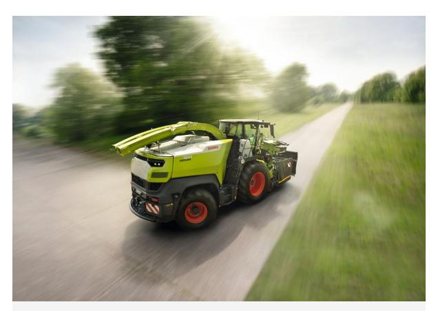
The discharge spout can be optimised for all PICK UP and ORBIS working widths. For harvesting with the new ORBIS 10500 with maximum manifold length, the end piece can be folded hydraulically for safe road transport.
