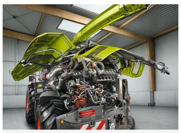
The JAGUAR 1080, 1090, 1100 and 1200 are powered by an efficient, transverse-mounted MAN V12 with a displacement of 24 litres. The innovative drive concept for the drives has been integrated into the overall concept to save space, resulting in an identical external width to the JAGUAR 800 and 900 and excellent visibility to the rear.
