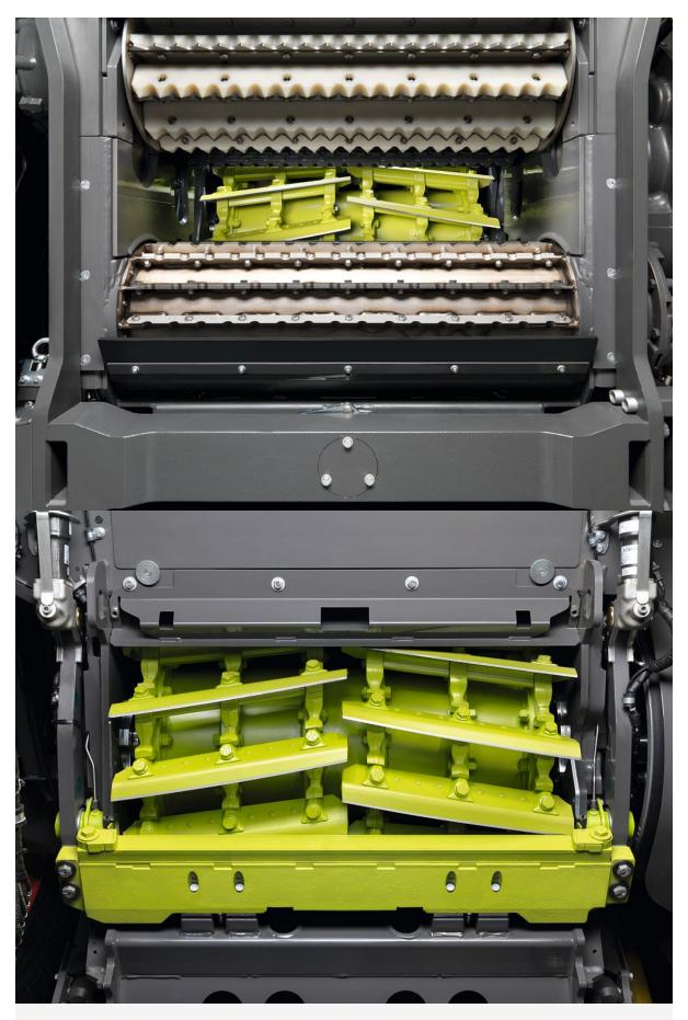
With a width of 910 mm, the V-FLEX chopping cylinder stands for maximum, continuous and blockage-free crop flow, even with the thickest swaths and in difficult harvesting conditions.
