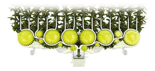
ORBIS 9000 and 10500 were specially developed for the JAGUAR 1000. The independent variable drive of the knife and transport discs as well as the feed drums allows optimum adaptation to the harvesting conditions.
