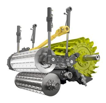
The pre-compression rollers ensure a uniform crop flow regardless of the layer thickness thanks to the new, fully hydraulic pre-compression system. The pre-compression unit can be swivelled open by 80 degrees for maintenance work.
