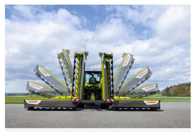
The new DISCO 9300 C / RC COMFORT offer exceptional operator comfort, especially in terms of hydraulic functions. The RC version is optionally available with the innovative double roller drive with scissor gear unit.
