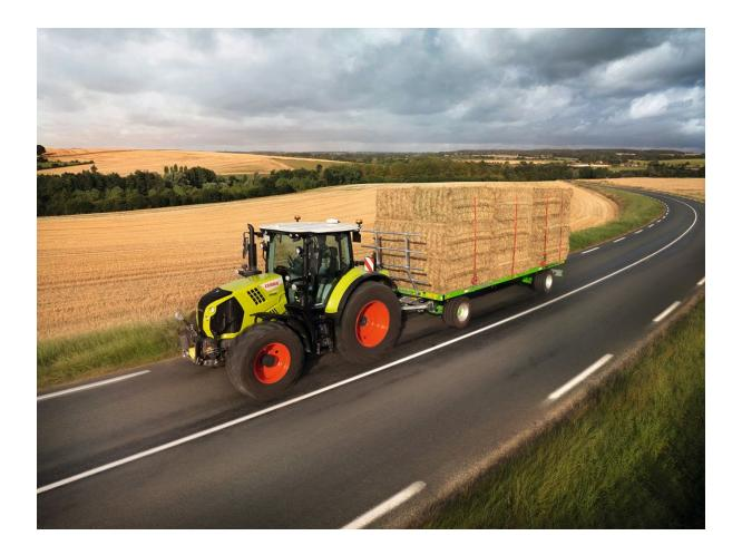
The automatic trailer stretch brake assists with transport operations and work with slurry tanks and balers on sloping sites.
