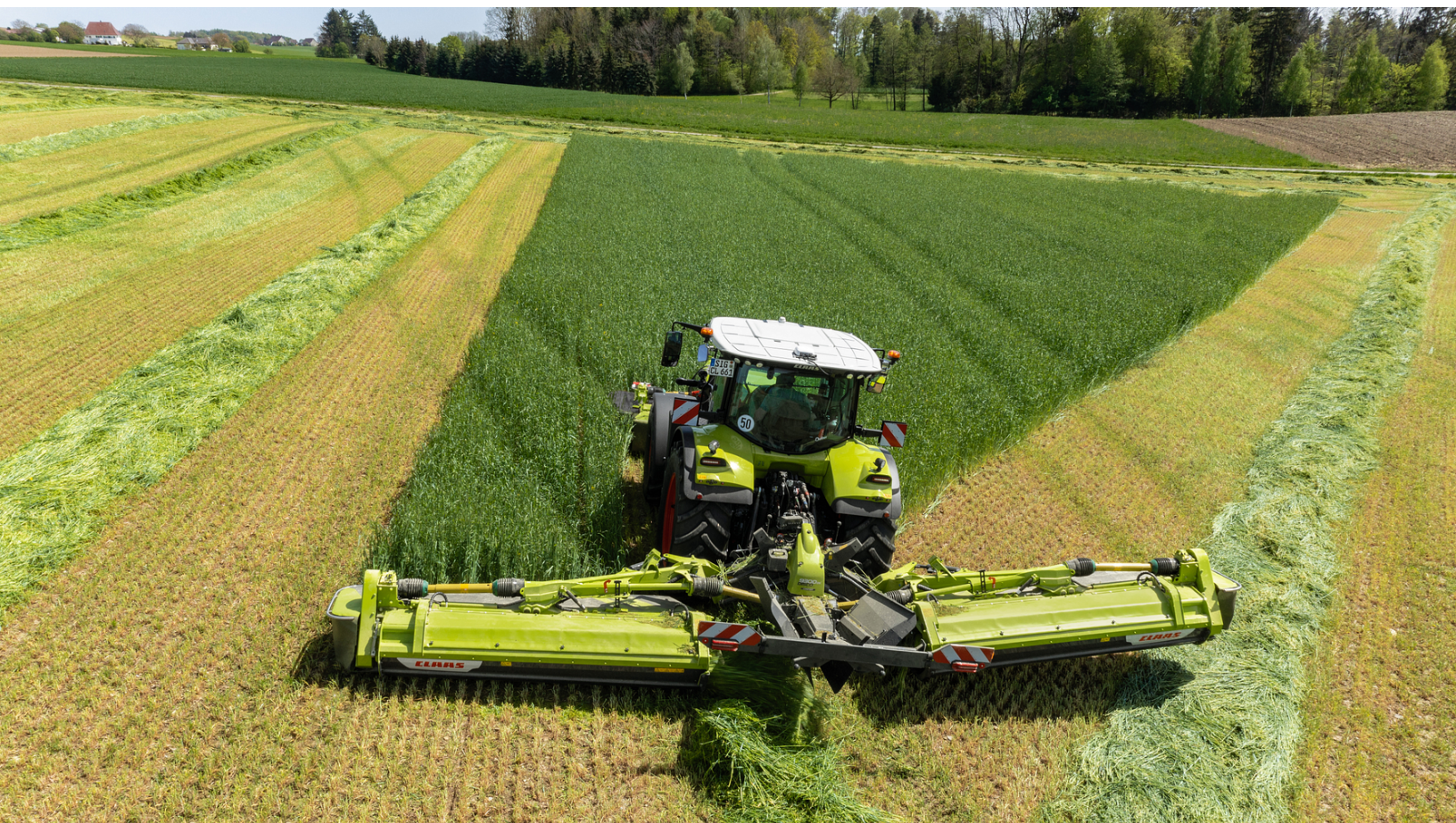
Flexible swath-laying via belt or auger
